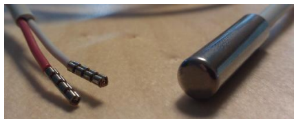
4pc sensors (supply and return line sensor, and the sensors for tap water)
